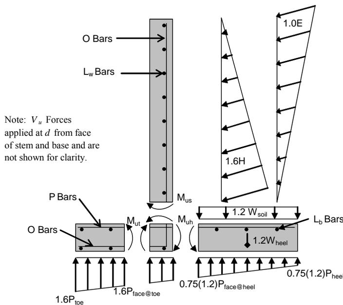
Figure 1: Reinforcing Bars and Element Loads
