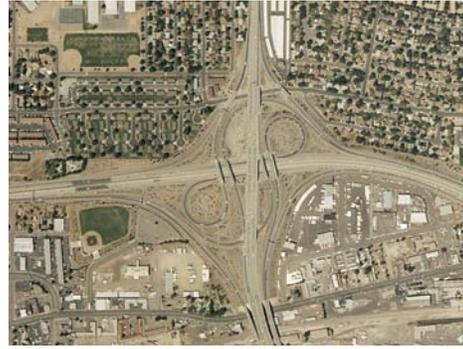
The Reno Bowl project was a \$60 million upgrade and improvement to the US-395/I-80 freeway. The project included widening and replacing over 6 miles of freeway structures, hydraulics, drainage, slopes and ramps and rehabilitation of over twenty structures, including seismic upgrades, bridge widenings several concrete and MSE retaining walls, over 6 miles of sound walls, storm drains and other miscellaneous structures.
