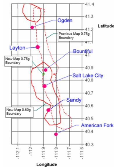
Figure 1 – Trigger Boundaries for Seismic Design Categorization from D to E/F
